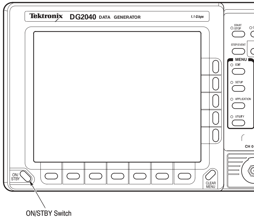
Figure 2-2: Location of the ON/STBY switch
